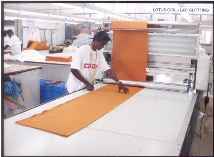
Spreader at Work
